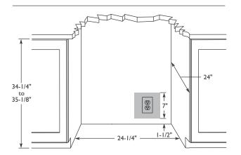
Follow the cut-out drawing The 24-1/4" width allows 1/4" for ease in installation and removal of the unit. 24" is the cabinet depth in most installations.
